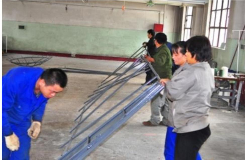
6) Making a semi-circle from one half of the wall supports. It should stand alone at that point. >
